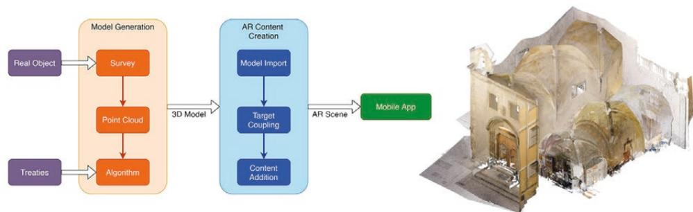
Fig. 1. Workflow from the survey to the mobile AR app (left); Point Cloud from the Laser Scanner surveys (right).
