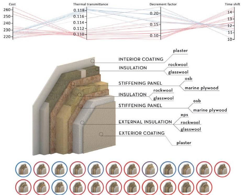
Fig. 1. The selection of various possible optimized walls according to thermal parameters, materials or cost.
